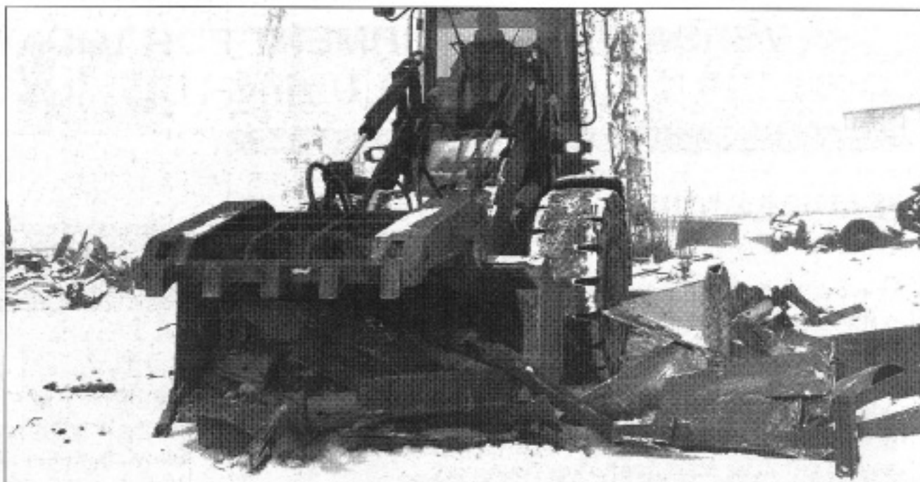
The Allied-Gator Claw Bucket is used to safely handle scrap where a normal bucket could not. The Claw Bucket closes on the scrap and actually compacts it, making it easier to handle.
